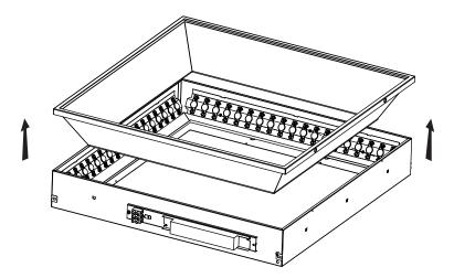
Remove 4 nos. screws from Diffuser Frame to open the Fitting for access.
